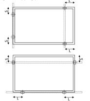
Fig. B: Clipping position on long & short frames
